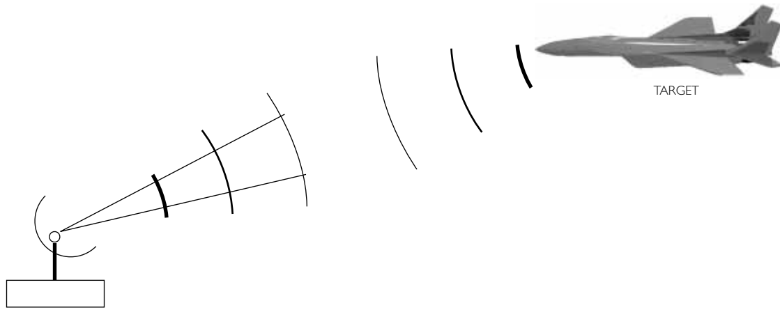
FIGURE 4: ECHO INTENSITY GETS SMALLER BY SIXTEEN WHEN RADAR TO TARGET DISTANCE DOUBLES
